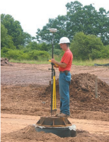
Sweeney's site superintendent, Pat O'Malley, uses Rover at manhole reference point to calibrate Base Station.
