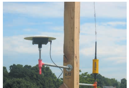
Above: Base Station and SiteNet radio are important components of SiteVision system.
